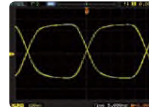
Rising & Falling Edge trigger Mainly used to view special signals such as eye-diagrams, formally only available in more advanced digital oscilloscopes
